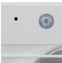
Model provided with a PIR (passive infra-red) detector. The unit starts automatically when a movement is detected within a maximum distance of 4 meters from the fan. They are also fitted with an adjustable "run on" timer, from 1 to 30 minutes, to allow the fan continues operating after the initiation of the movement detection.
