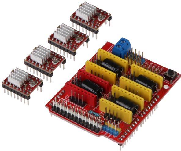
With this expansion board, which is made for use with an Arduino Uno or Arduino Uno compatible board, you can install a custom CNC router. It can be powered from 12 to 36 volts depending on your needs. Control with the four included A4988 motor drivers operates up to 4 axes and is lightweight as it is 100% GRBL compatible.
